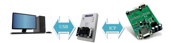
Step 1: Test and save the project (\*dprj) under Dediware engineering mode. Make sure you select "Start from handler" for start mode in the Config window.
