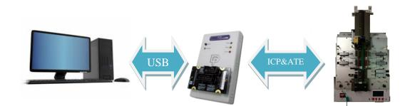
**Step 1:** Test it under Dediware engineering mode, and then save the project file as \*.dprj. Use **start mode** to set-up the handler. And use DownPrj to load the project file to the embedded memory.
